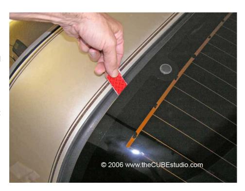
**RESTORATION TIP:** You may find that the factory has done a crappy job of cutting out the slots in the panels which will have the hinges rubbing when the glass is open. Carefully remove the rubber trim piece and cut the slot straight as shown:
