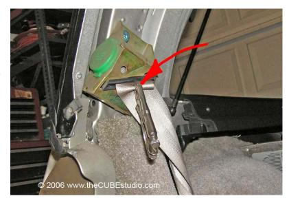
4) With the hatch closed, remove the old hinges from the car . . . note that I will refer to this part (shown in the next picture) as the 'glass button'. It is made of steel and has a smaller diameter 'barrel' that reaches thru the glass and into the hinge. It has two plastic washers; one that you see under the button (this one reaches thru the glass), and one plain flat washer on the under side that goes between the hinge face and the glass surface:
