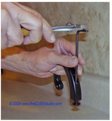
The above technique works to get the original stuck buttons out during disassembly, but be very careful if you are tapping on the allen wrench (or pin punch) to get a button loose while the hinge is still installed as the glass is taking the shock of the tapping.
