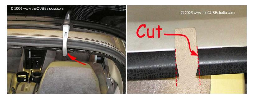
**10)** Open the glass and install the struts. The tube end goes UP (toward the back of the car when the hatch is closed).
