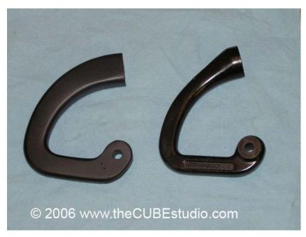
Note that if you received your hinges prior to November of 2007, the punch marks face the inside. To make the punch marks easier to see during installation, I began placing the punch marks facing toward the OUTSIDE of the car after that.
