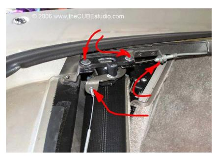
The other side has a similar latch, but both cable adjustments are on the left side hatch shown. The cable adjuster (on the right in the photo) is for the pull handle, and the other one is between the latches and is used to adjust the latches to open at the same point.
