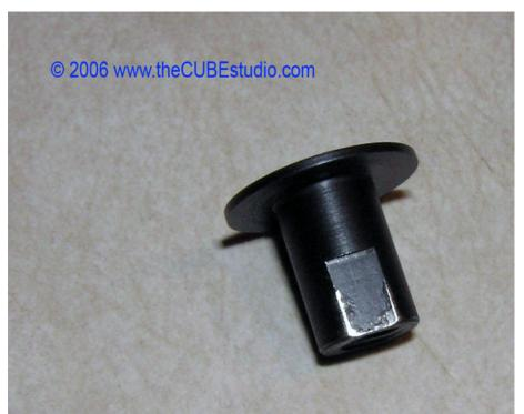
Knocking that sharp edge off should cure the snug. But the bolt will pull it in no problem without modification, as was done in the example shown in the above photo.
