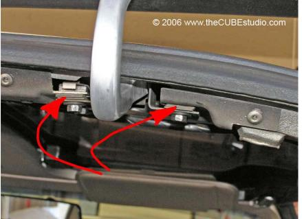
one body to the next in C3 corvettes. I believe there is also 'replacement' glass and I know there is 'replacement' weather strip. This adds up to a lot of variation from car to car. There is a lot of adjustment available in the hinge mount so you should be OK. At this point the hinge mounting bracket should be fairly well aligned with the car body mount. It should be parallel and need a few shims like this picture shows. If not, something is wrong so please STOP and contact me.
